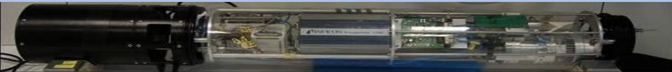
Analyzer unit MIS & Gear pump Sample inlet
