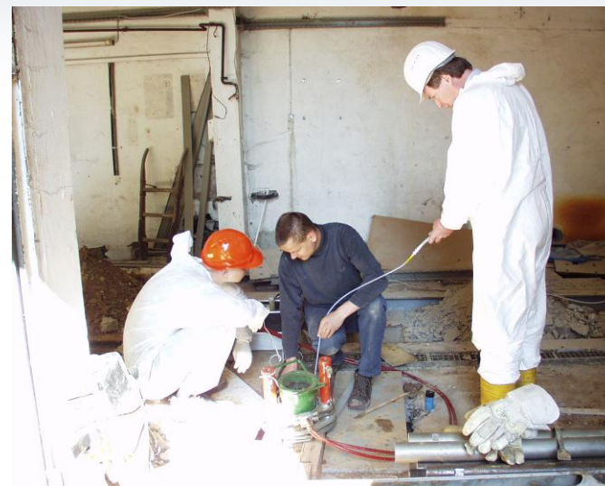
Sampling of ground air (down to 7 m)
