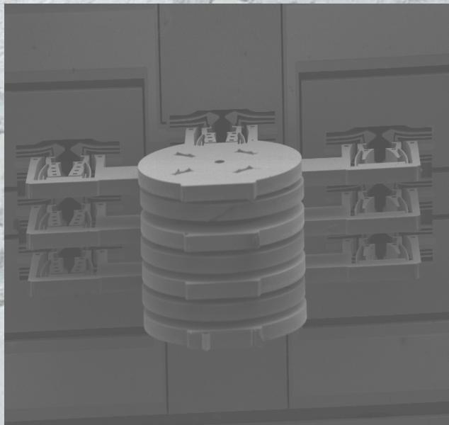
SEM image of the Coaxial Ring Ion Trap with 500um i.d.
