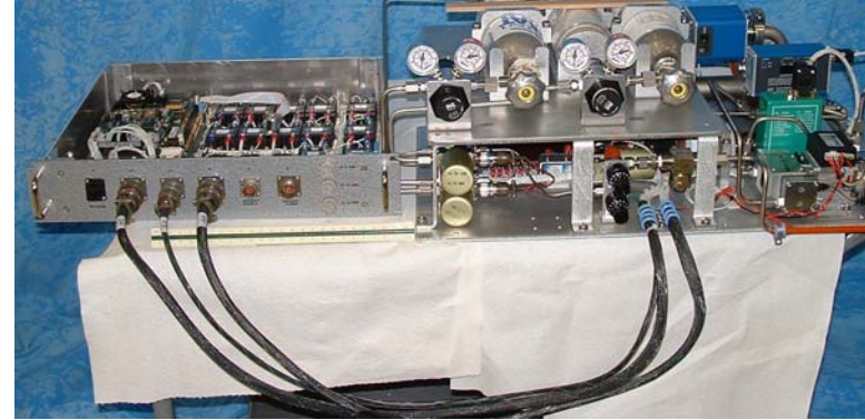
AVEMS (Primary Mission Instrument) Airborne Volcanic Emission MS System KSC-NASA (RGA 200)- Autonomous
