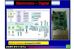
We have developed an imbedded micro computer, using an ARM 9 CPU. The printed circuit board is a 7 layer board with more than 5000 connections.
