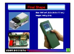
All integrated final shape looks like this. The size is  $8.2 \times 24.5 \times 7.7$  cm and the total weight is 3 pounds. Battery weight is excluded because you can use a various size of batteries. If you use 400 g battery then the operation last about 10 hours, and 200 g battery then 5 hours.
