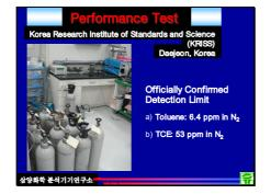
The PPMS was officially tested by Korea Research Institute for Standards and Science. The officially confirmed detection limit is 6.4 ppm for toluene in the air and 53 ppm for TCE.
