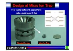
This picture compares the size of the standard ion trap and the micro ion trap used in the PPMS. It is consists of four parallel plates with coaxial holes that makes a quadrupole electric field inside virtually the same as that of standard ion trap
