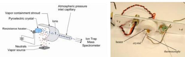
Schematic and photo of ion source. Ions are produced at the  $-z$  face of a pyroelectric crystal and travel through the vapor containment shroud to the atmospheric pressure inlet capillary of the mass spectrometer. The crystal is heated by a resistor cemented to the  $+z$  face.
