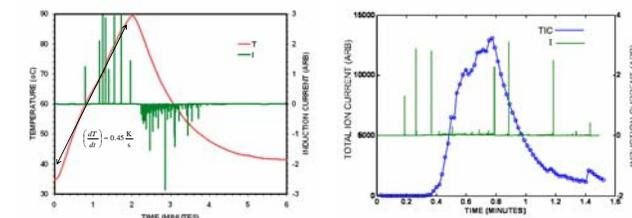
Electrical discharges are observed during heating and cooling. An inductive pickup monitors discharges as the temperature changes (left). Most ions are produced during periods of apparent electrical quiescence (right). Visible discharges are observed which correlate with the surges in induction current.
