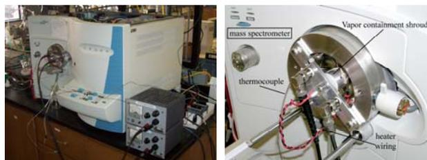
APPIS source mounted on ThermoFinnigan LCQ Deca XP ion trap MS.
