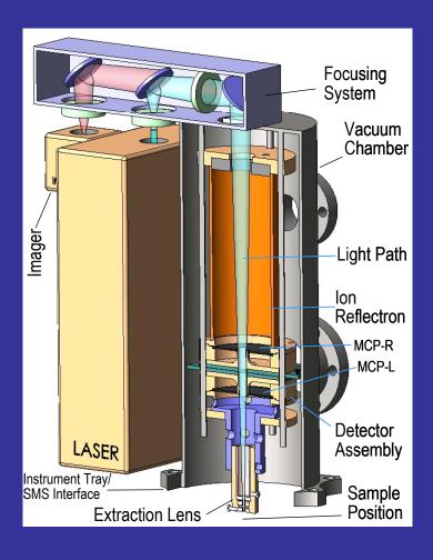
Sensor is ~ 50% size of DS-TOF prototype, and mounts on 450CF flange. Flight model bundles laser and microscopic imager in common optical system.
