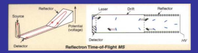
The reflectron corrects TOF dispersion: ions with same m/z but different energies arrive at the detector simultaneously. A nonlinear reflectron focuses LA and LD ions (wide KE band) as well as organic product ions.
