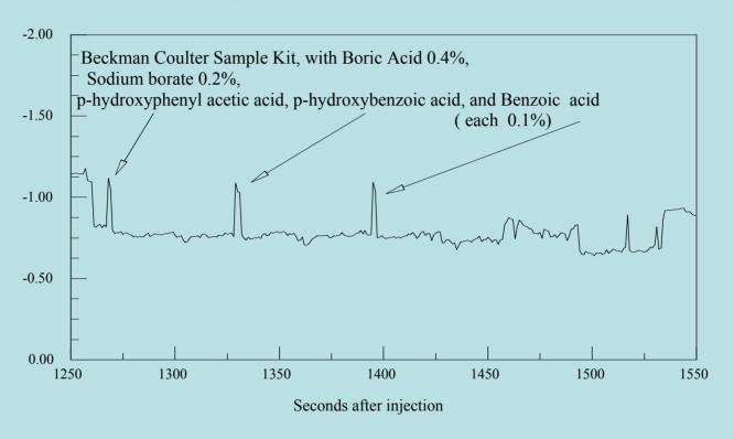
*Figure 24.* Capillary Electrophoresis demonstration of Mass SURFER sample inlet. Four sharp peaks are detected, the first three of which are identified and labeled.
