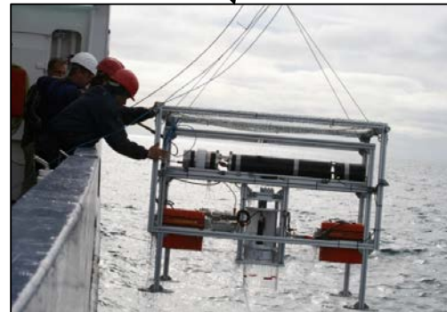
In situ in a frame including benthic chamber
