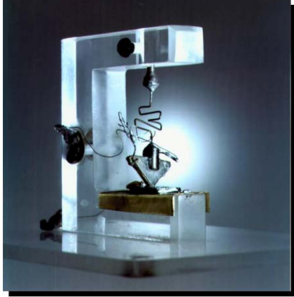
1947 The First Transistor from Bell Labs
