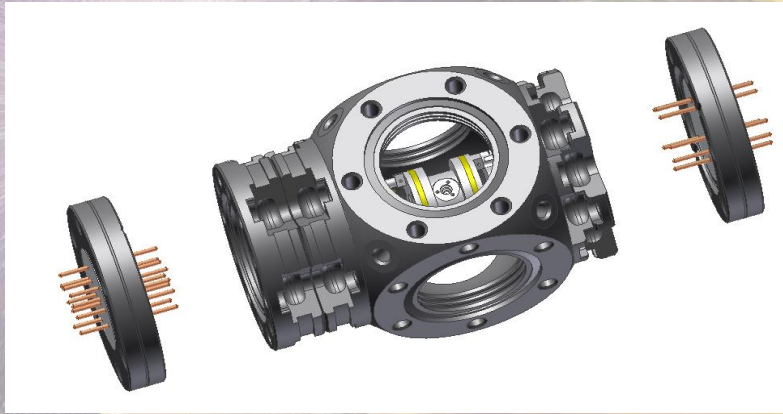
T3: 4.5 mm trap in 2.75" spherical cube
