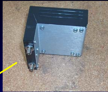
Resistively-heated LTM GC column
